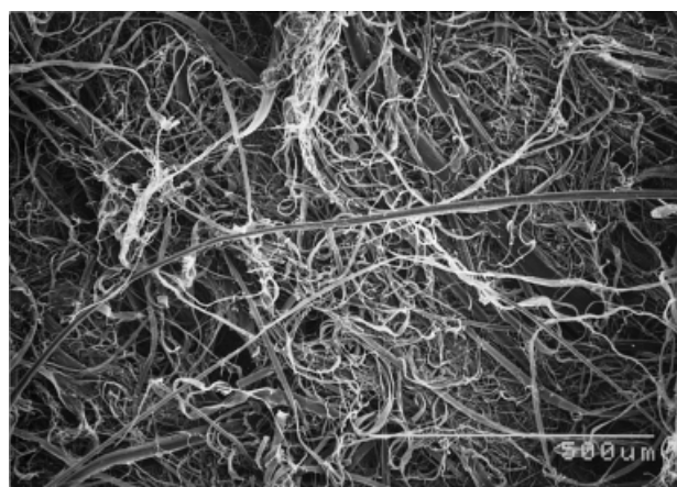
Figure 5 SEM micrograph of pulp-shape PAN fiber obtained by pulping the porous PAN fiber.
